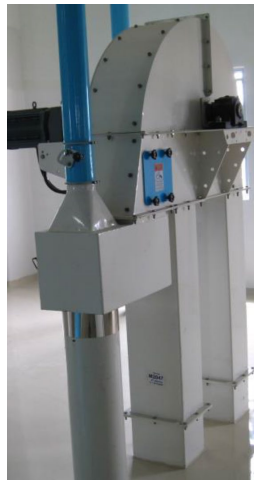
Boot + head exhaust arrangement for bucket elevator
