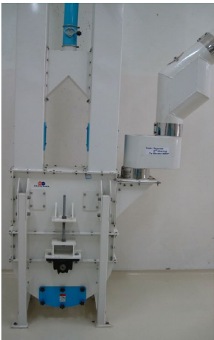
Boot + head exhaust arrangement for bucket elevator
