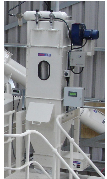
Micro tip station filter arrangement
