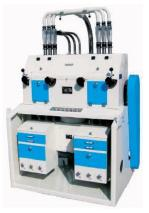
The Pilot Mill is a fully automatic laboratory test mill for rapid milling of production equivalent test flours. Multiple grinding is carried out by fixed corrugated rolls. The separation of the products is achieved in a two-section sifter. The flours produced by this machine are equal to those obtained on a commercial mill.
