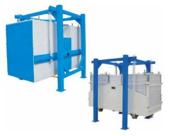
The Twin-Section Plansifter is a compact and light-weight machine which can be easily installed anywhere. It is suited for product grading in a wide variety of industries, such as flour milling products, feed milling products, maize milling products, foodstuffs and products of the chemical industry. Experience has proven the suitability, reliability, easy operation and minimum maintenance features contained in the machine.
