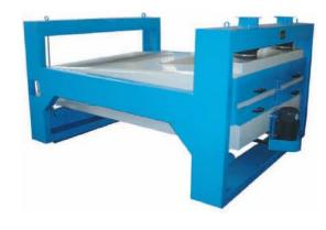
The Rotary Separator is used to separate foreign impurities of various dimension from a wide range of seed, cereal, pulses and similar granular products.
