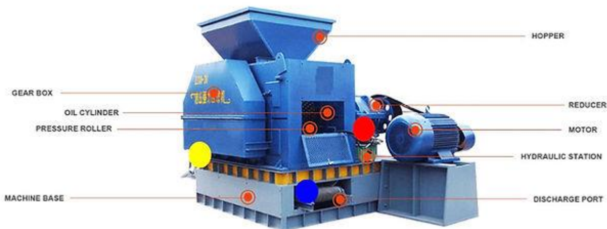
Structure of Briquette Machine
