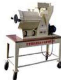
Abrading M/C 5XP-50 CAP. 50Kg/Hr
