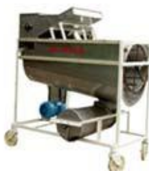
Indent Cylinder M/C 5XW-100 CAP. 100Kg/Hr
